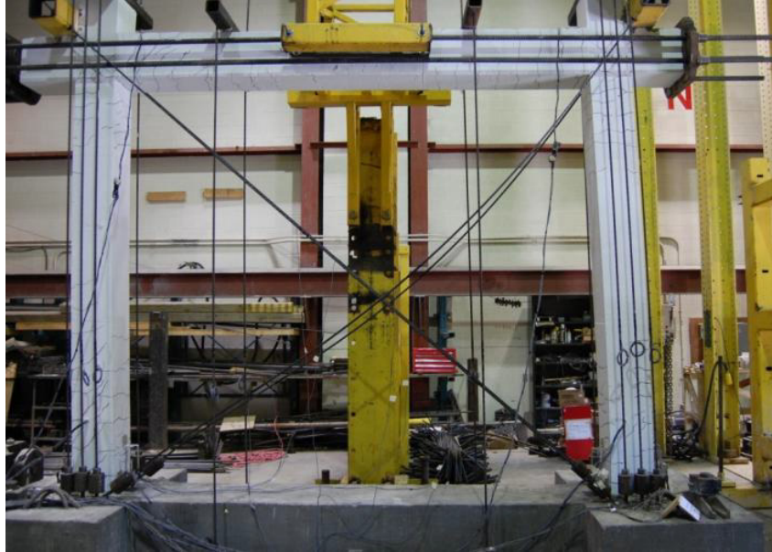
Fig. 4.10 Frame No. 2 at 1.75% drift during the pull cycle
