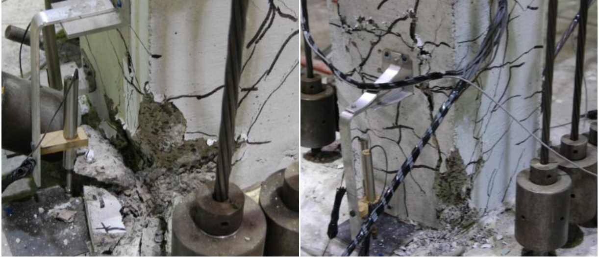
Fig. 4.5 Damage at column base at the end of 2.5% cycles (failure cycles)
