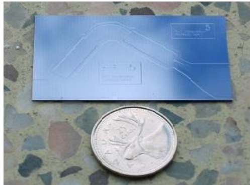
Fig. 3.1. An illustration of the AWG chip used in the thermal tuning wavelegnth interrogation unit.
