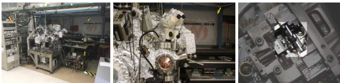
Figure 6.1: NRC's Omicron STM-1, STM chamber and scanning head. (a) Omicron STM-1. (b) STM chamber. (c) Scanning head with tip and sample highlighted.
