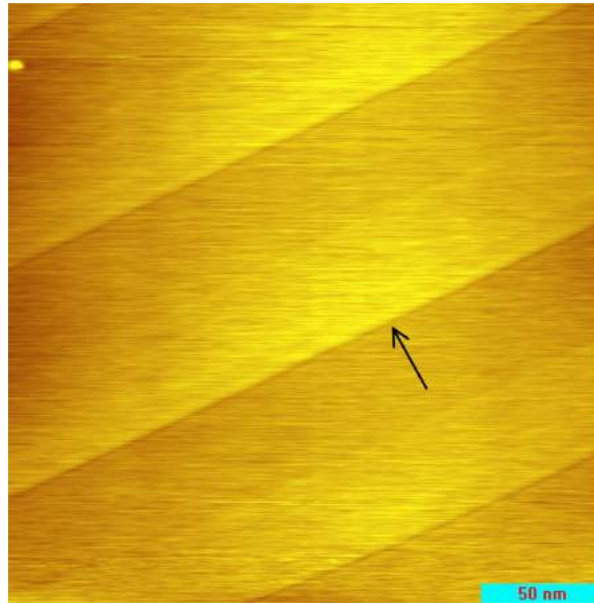
Figure 2.13: STM of graphite step edges. V_b=0.1\text{V} ; I_t=500\text{pA} . Size= 250\text{nm} . Taken with RHK STM.
