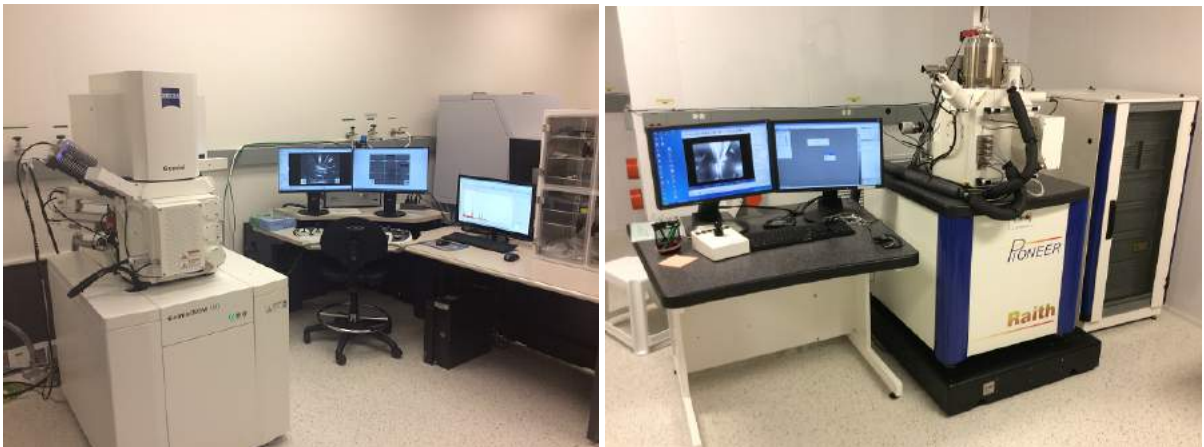
Figure 6.4: Scanning electron microscopes used for characterization and electron-beam lithography. (a) Gemini 500 SEM. (b) Raith Pioneer.
