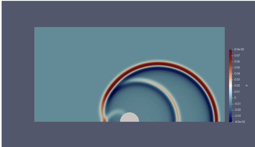
Figure 21: Pressure at t = 3 for the acoustic scattering off a circular cylinder case using the hp-adaptive immersed boundary implementation. Parameters as in Fig. 19.
