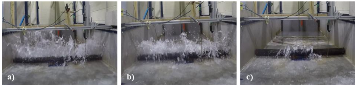
Figure 4.7. Bore impact on the pipe on the pipe for three impoundment depths: a) h = 50 cm, b) h = 40 cm and c) h = 30 cm.
