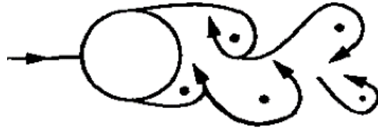
Figure 2.4. Laminar 40 < Re < 200 and turbulent 200 < Re < 350 vortex shedding. (Adopted from Sumer and Fredsøe 2006)
