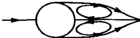
Figure 2.3. Attached eddies, 5 < Re < 40 . (Adopted from Sumer and Fredsøe 2006)
