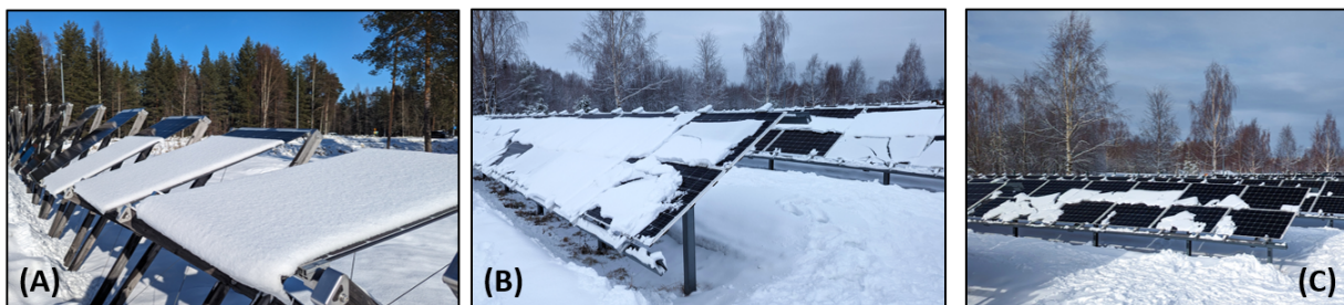
Figure 4.13: Images of snow shedding patterns on bifacial PV modules. Photos taken by the author for (A) Piteå Solvåg and (B-C) a Luleå Energy PV plant.
