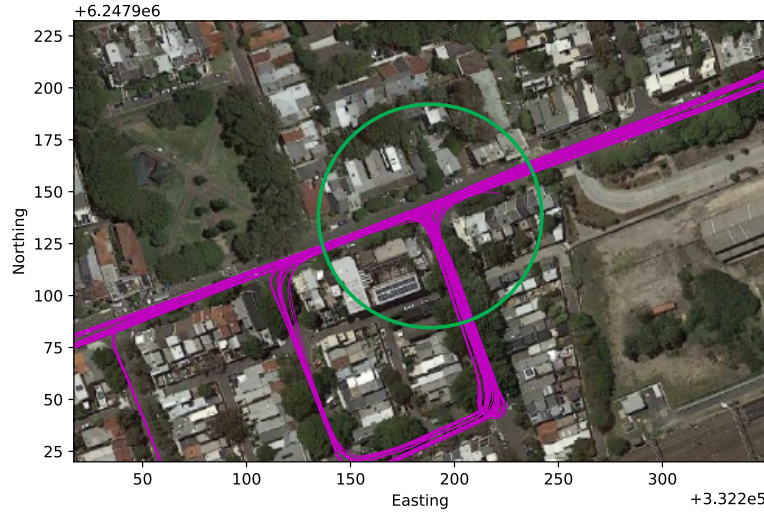
Figure 6.1: A sample of vehicles trajectories within the unsignalized T-junction.
