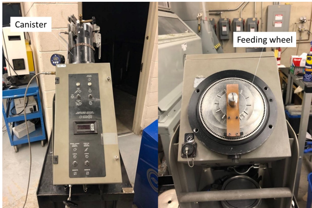
Figure 44. Powder feeding canister (left) and feeding wheel (right)
