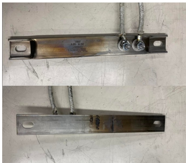
Figure 46. Strip heater beneath (top) and conducting side (bottom)
