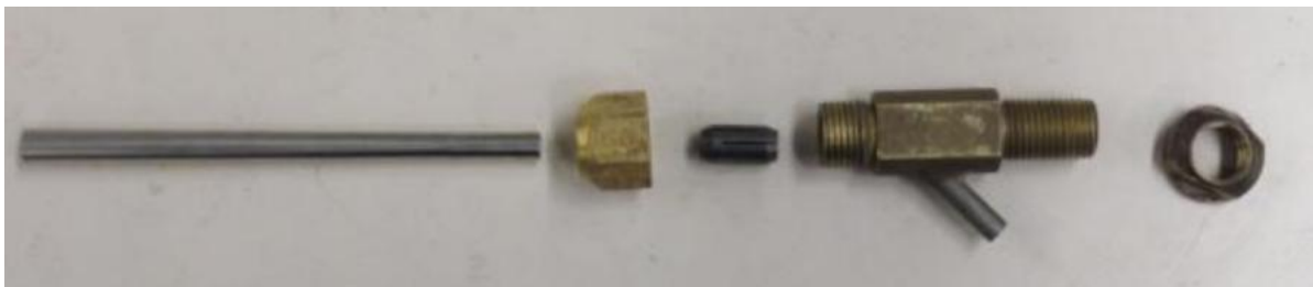
Figure 80 Disassembled de Laval Metal Nozzle Showing, From Left to Right, Stainless Steel Nozzle, Tightening Nut, Tightening Collet, Brass Orifice and Heater Nut [111]
