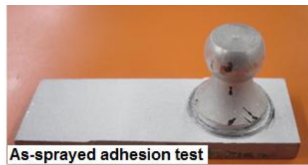
Figure 102: Pull-stub Glued to Coating
