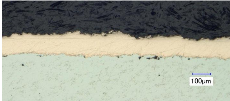
Figure 164: Cross-sectional View of Copper Coating on Invar Mould Pre-treated with Nitric Acid.
