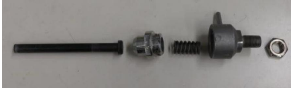
Figure 81: Disassembled de Laval Plastic Nozzle Showing, From Left to Right, Plastic Nozzle, Quick Connect Cap, Spring, Orifice and Heater Nut [111]
