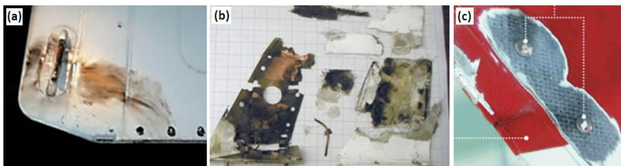
Figure 5: Damage Resulting from Lightning Strike for a (a) Horizontal Stabilizer, (b) Antenna and (c) Riveted Composite Trailing Edge [5]
