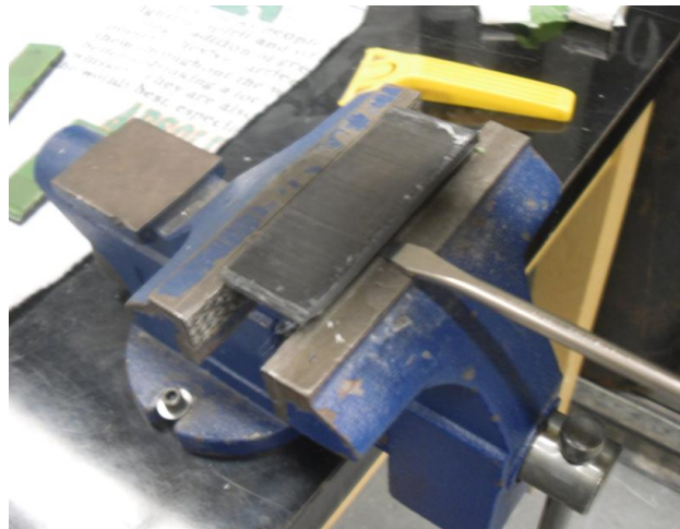
Figure 90: Metallic CFRC Removal Method
