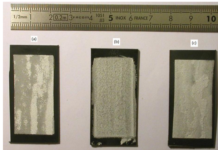
Figure 17: Delaminated Aluminum on Polyamide 6,6 Substrate using (a) T_{\text{gas}}=150^{\circ}\text{C} (b) T_{\text{gas}}=300^{\circ}\text{C} and (c) P_{\text{gas}}=3 \text{ MPa} [32]
