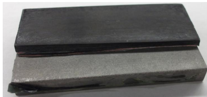
Figure 91: Removed Metallic Composite from Mould
