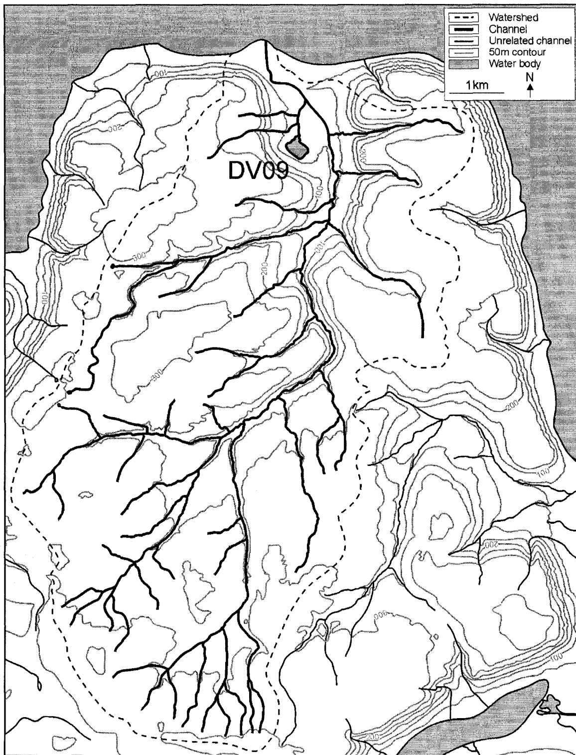
Fig 1.4: Map showing the drainage network that DV09 is a part of, yet has no direct input streams. Adapted from 1:50 000 NTS maps 58 H/07 and 58 H/10.
