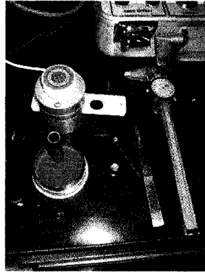
Figure 4.7: The procedure and tools for extracting the specimens for the psychrometer measurements
