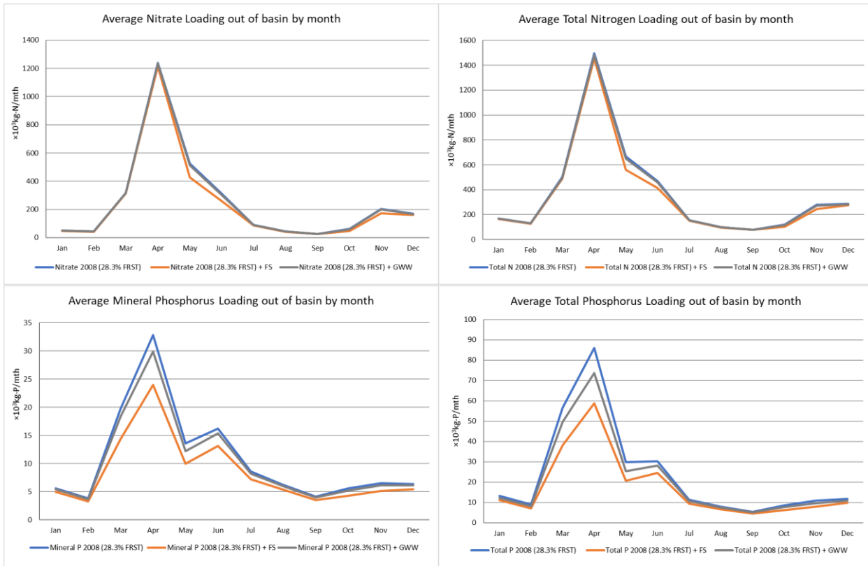
Figure 27 Monthly average exports of sediment and nutrients from the basin, 2008 LU scenario with and without BMPs simulated
