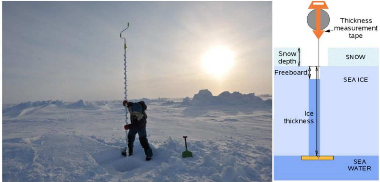
Figure 2-9: Drilling into Sea Ice (left) (Hartley, 2022) and Augur Fast Ice Measurement Schematic (right) (Mahoney & Gearheard, 2008).
