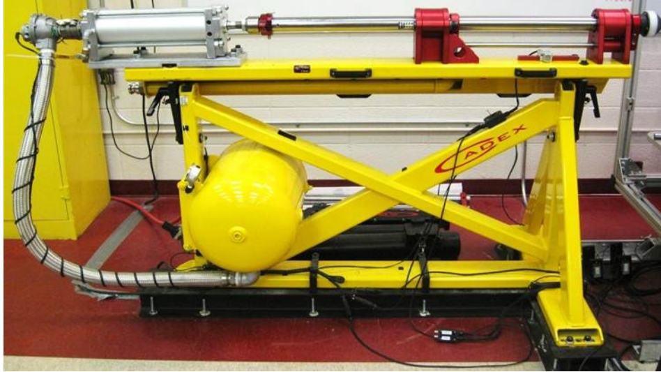
Figure 2: Pneumatic linear impactor with pointed impactor striker
