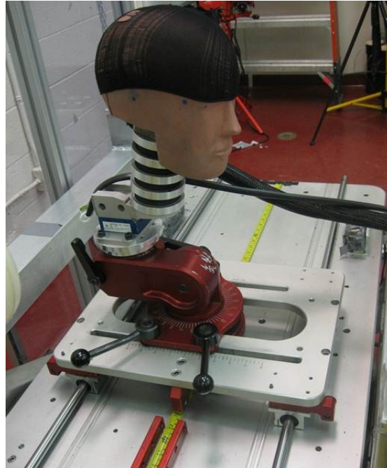
Figure 6: Sliding table with Hybrid III head and neckform attached
