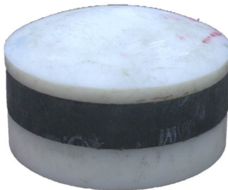
Figure 1: Large modular elastomer programmer pad (MEP) striker
