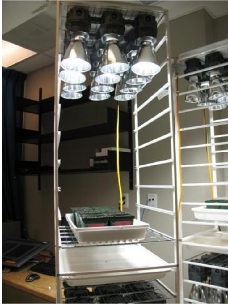
Figure 13: Light shelves used to grow plants in pots (green) in the lab also called ArabiSun.
