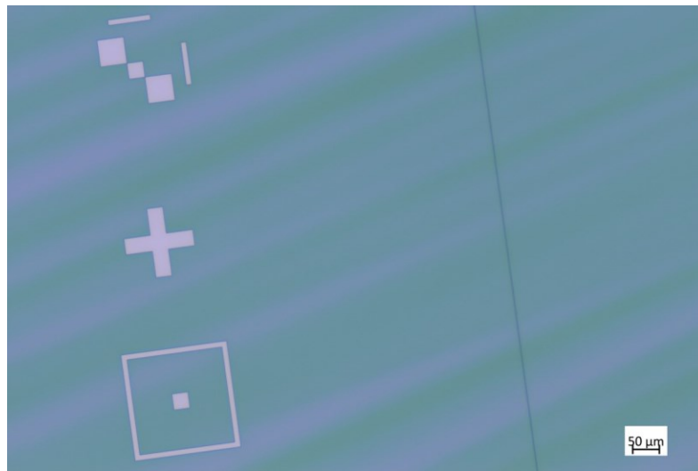
Fig. A.4 An optical microscope image of a region on the wafer at the end of Step A.1.2, showing the developed photoresist patterns after the first photolithography process.
