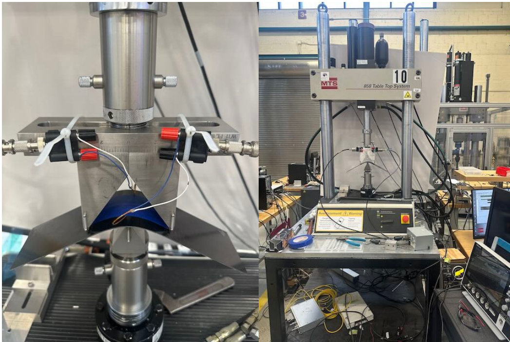
ESI 3.7: Laminate 2 during 3 point bend test (Left). Final setup for 3 point bend test (Right).
