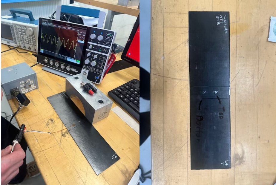
ESI 3.6: Initial setup of sensors for 3-point bend test, including the oscilloscope, switch, and function generator (Left). Laminate 4 before stress testing (Right).
