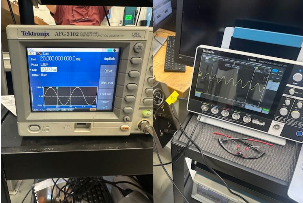
ESI 3.8: Picture of function generation during 3-point bend test (Left). Picture of oscilloscope during 3-point bend test (Right).
