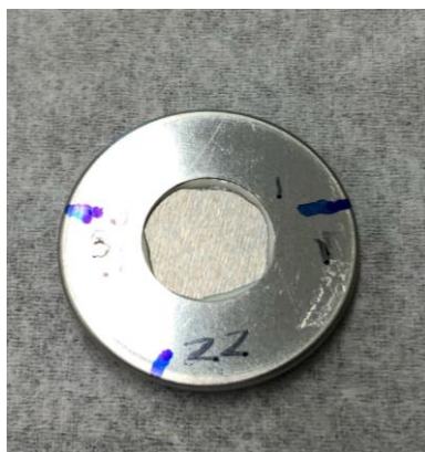
Figure 3.4.3. Single-use beryllium window coin-cell for operando XRD
