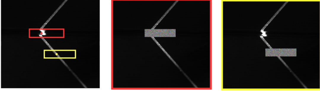
Figure 4.4: Modification of input images for the cutout discriminator networks based on the keypoint c_m and a random offset \Delta d_m . Red frames correspond to positive samples while yellow show negative samples.
