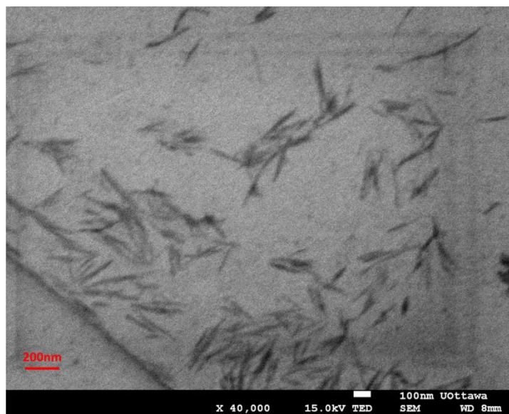
Figure 3.3 TEM image of CNC particles
