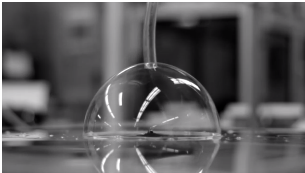
Figure 2.3: Blowing the soap bubble with hydrogen-air.
