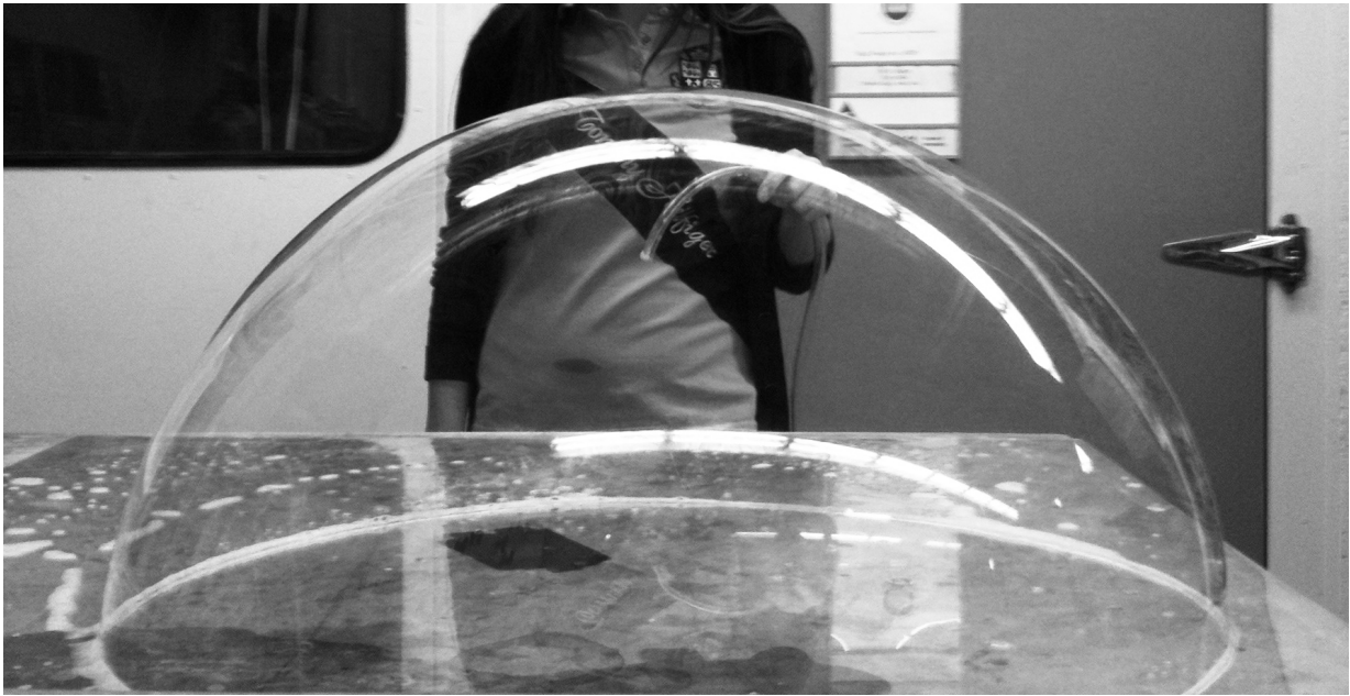
Figure 2.7: A 63.5 cm diameter bubble made using the guar solution.
