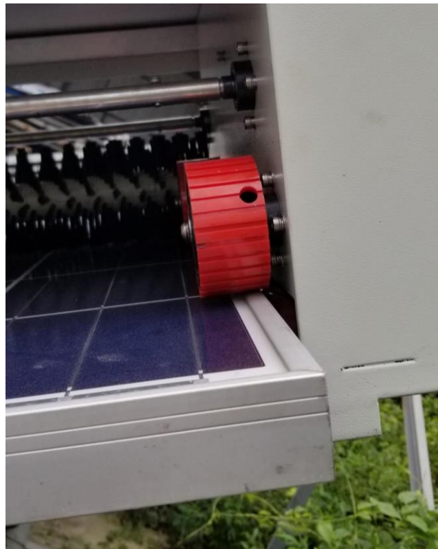
FIGURE 4.6 Robot wheel riding on the solar panel frame.
