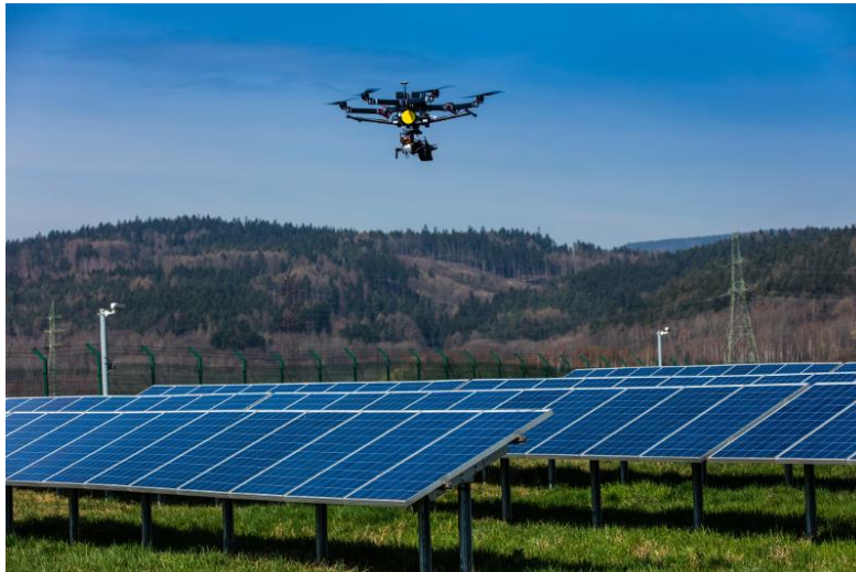
FIGURE 1.9 Drone with thermal camera performing “hot spot” inspection. [53]
