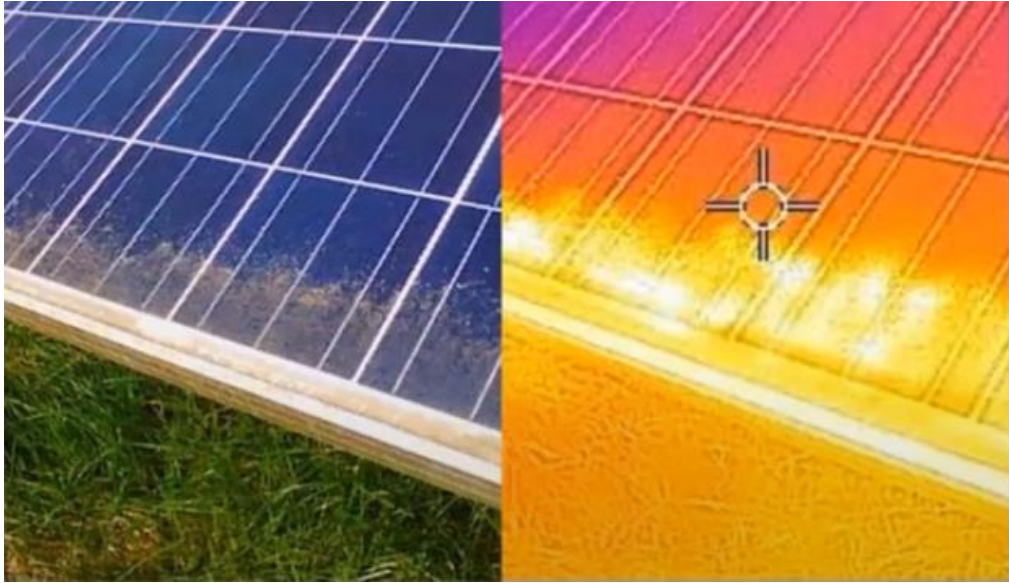
FIGURE 1.8 Shading causes “hot spot” on solar panel. [52]
