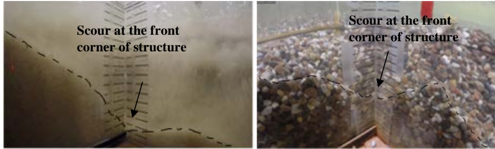
Figure 7-9: Final scour profile from the inside video camera a) sand - dry condition, b) gravel – dry condition
