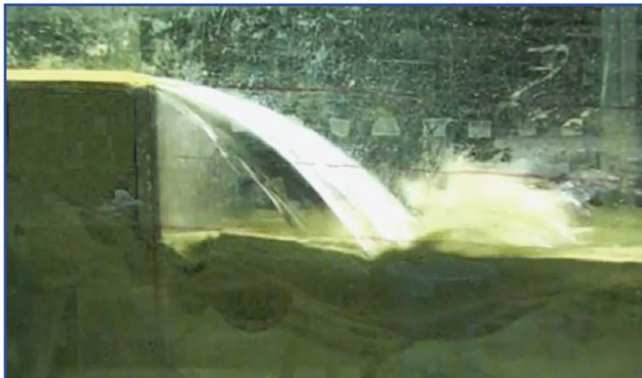
Figure 2-12: State from which the scour by a back-flow started
