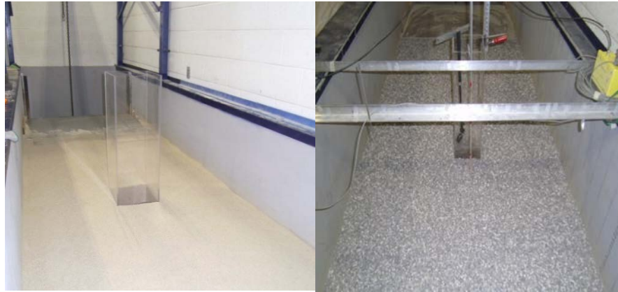
Figure 7-2: Sediment section: Left: Sand bed, Right: Gravel bed
