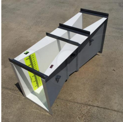
Figure 9: Parshall flume measuring structure, uninstalled [34].
