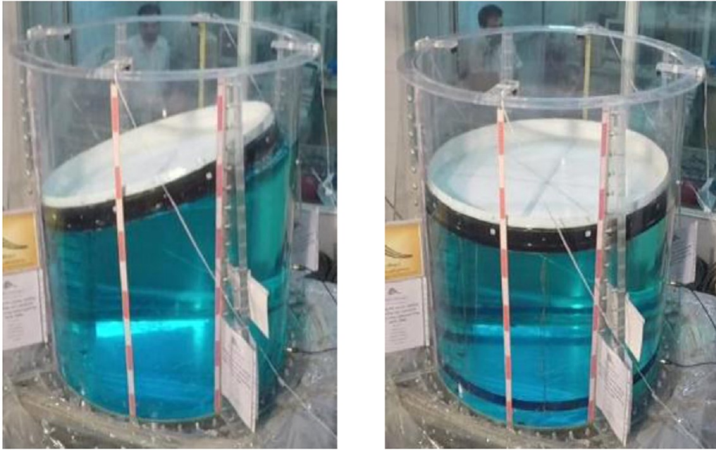
Figure 23: Experimental study of an annular suspended baffle, Hosseini et al. 2017
