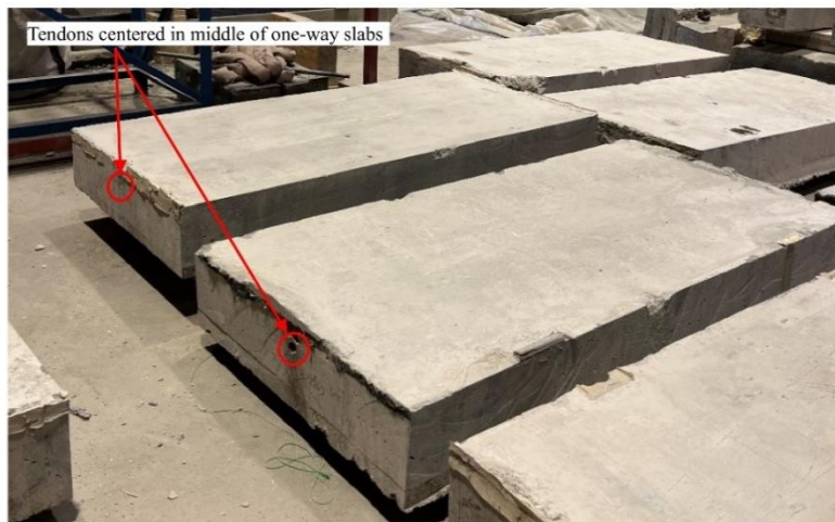
Figure 4-4 Full-scale prestressed concrete slab specimens prior to testing (inverted)
