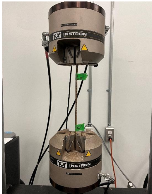
Figure 5-6 Tensile test set-up
