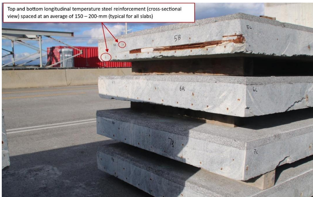
Figure 3-3 Stacked infill deck slab samples (transverse edge)
