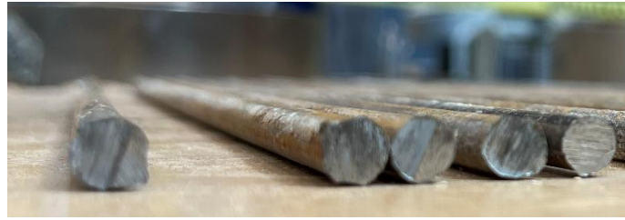
Figure 5-4 Control wire samples obtained from diaphragm segments
