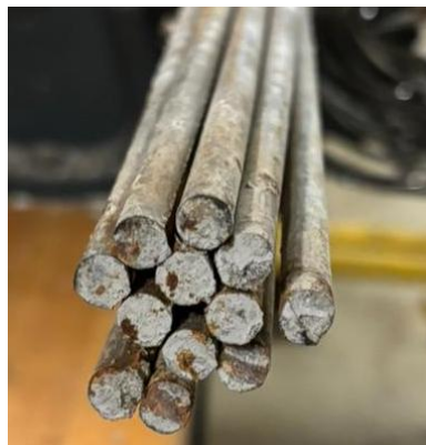
Figure 5-5 Isolated wires from a single post-tensioning tendon
