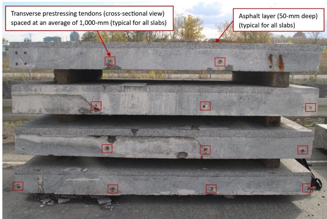
Figure 3-2 Stacked infill deck slab samples (longitudinal edge)
