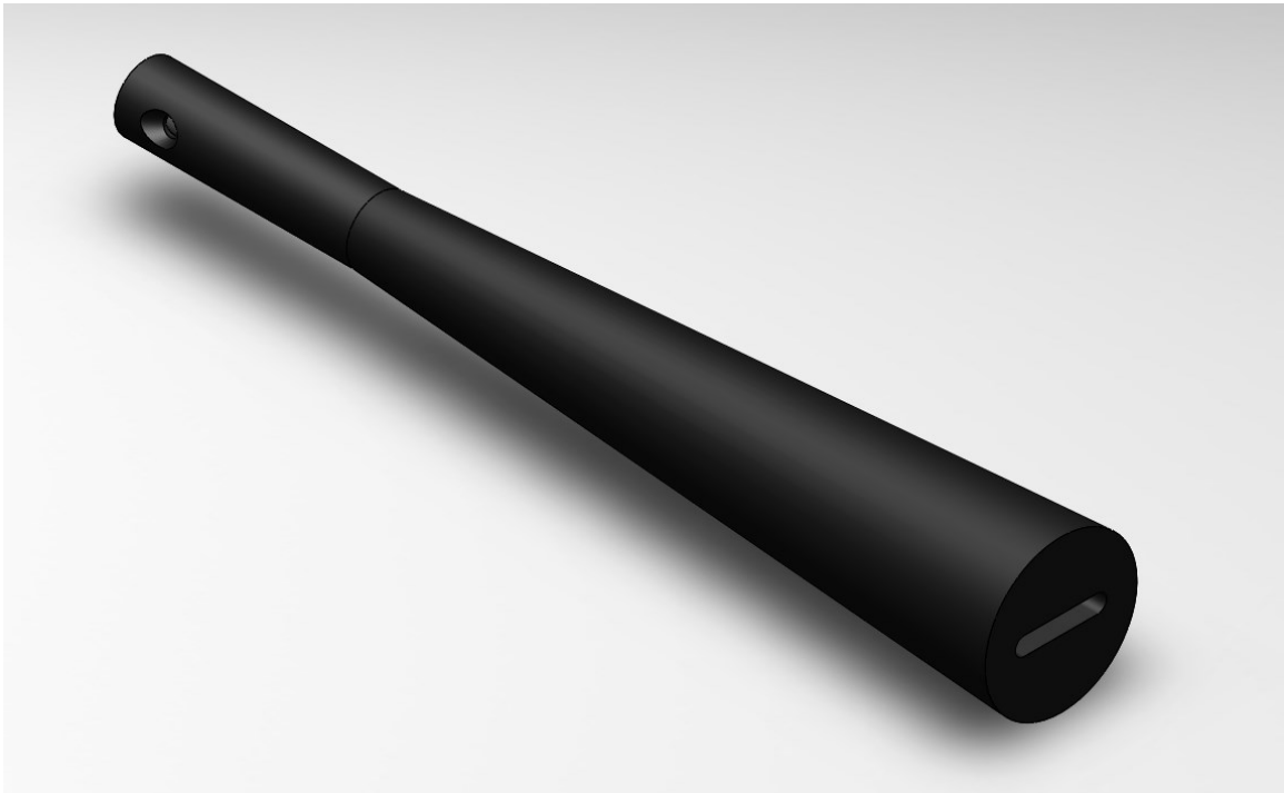
Figure 5.20 – CAD model of the initial angled (15°) injection obround prototype
