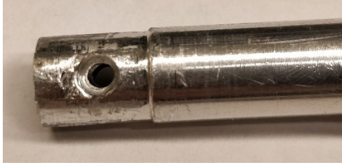
Figure 5.30 – Second powder inlet on the obround PBI nozzle prototype
