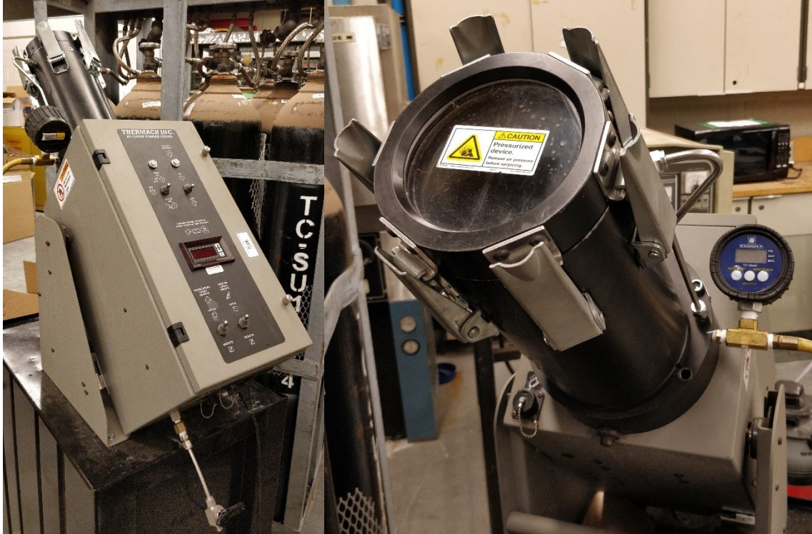
Figure 4.10 – Secondary powder feeder and alternate view showing the pressure vessel where the powder is contained
