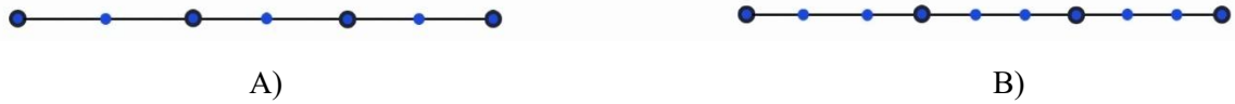
Figure 4.1: Example of p -uniform refinement on a uniform mesh with three elements. (A) corresponds to polynomial degree 2, while (B) corresponds to polynomial degree 3. The blue points indicate the additional nodes introduced by the higher-order basis functions.
