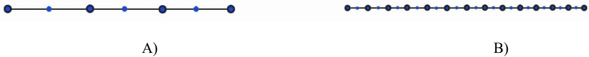
Figure 4.2: Example of h -uniform refinement. In (A), the mesh consists of three elements with polynomial degree 2. In (B), the mesh is refined into 13 elements while maintaining the same polynomial degree 2.
