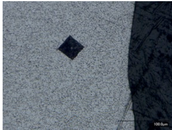
Figure 51: Optical micrograph of the etched screw sample illustrating deformed grains at surface layer
