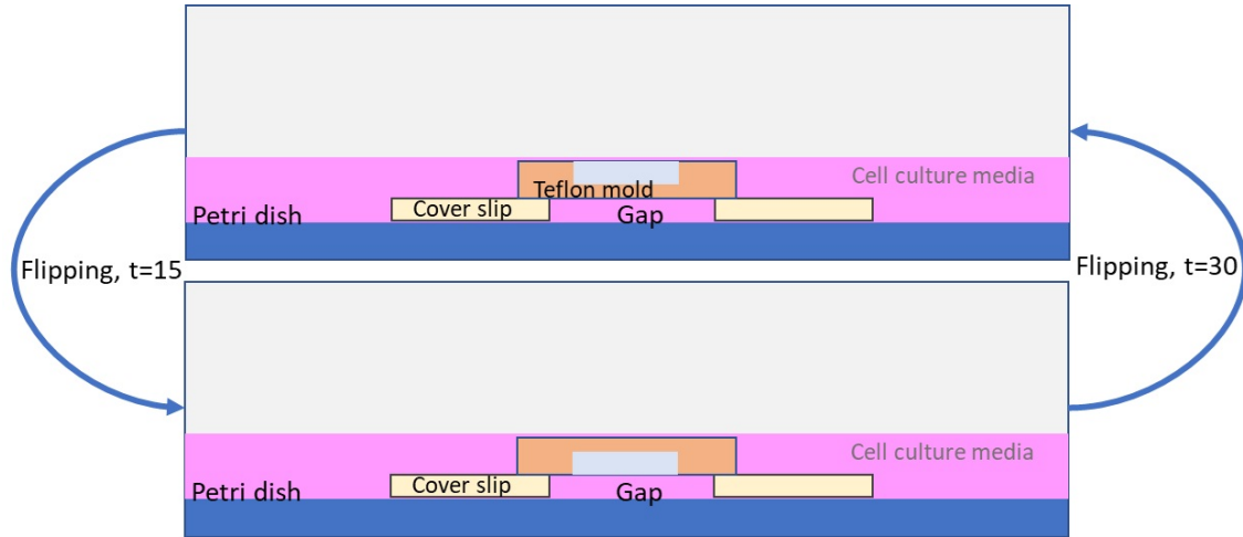
Figure 3.1: Flipping process Schematic representation of the flipping process used to ensure homogeneous cell distribution within the collagen scaffolds.
