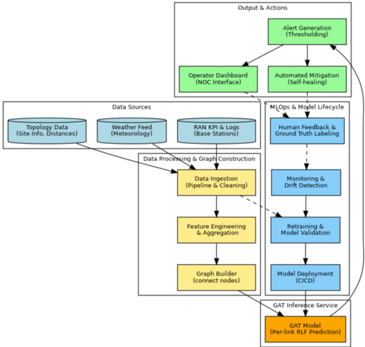
Figure 4.5: End-to-end pipeline for GAT-based RLF prediction: data sources (topology, weather, KPIs/logs) → ingestion/cleaning → feature engineering → graph construction → GAT inference (per-link failure probability) → thresholded alerts for NOC dashboards and automated mitigation, with an MLOps loop for monitoring, feedback, retraining, and CI/CD deployment.
