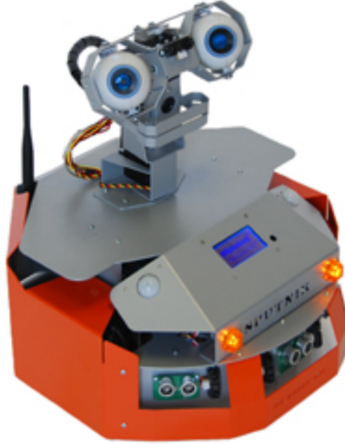
Figure 7.11: Sputnik mobile robot used for tracking an U-shaped trajectory in the MIRaM laboratory.
