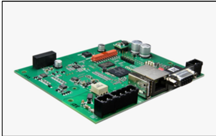
Figure 3-1: EVCharge SE Board [ELE]
