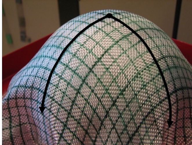
Figure 5-5 Laboratory Drape on the Hemisphere With Start Point and Geodesics [72]
