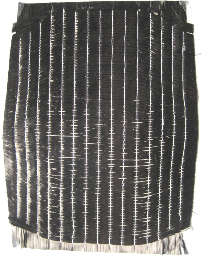
Figure 5-29 Manufactured Textile for the Aerospace Mould Optimised for Surface Area
