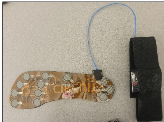
Figure 7.5. Smart insole to capture plantar pressure
