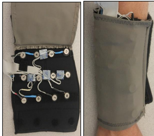
Figure 7.6. Haptic armbands to send vibrotactile signals for athlete training
