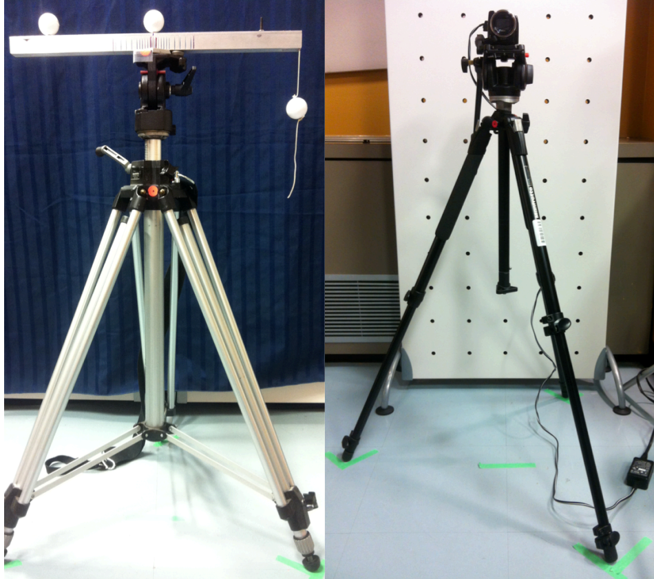
Figure 1. Experimental set-up for accuracy and reliability testing. The photo on the left is the sliding aluminum rail mounted with spherical markers, and a hanging ball on the right. The photo on the right is the camera, set up perpendicular to the apparatus.
