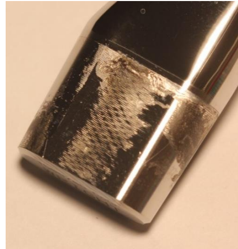
Figure 4.14: Severe wear on the anterior surface of an impact-assembled Ti6Al4V neck following a fatigue test leading to material removal off the neck taper.
