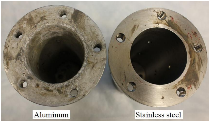
Figure 3.9: The effect of the corrosive testing environment at the top of the inner edge of the aluminum specimen holder.
