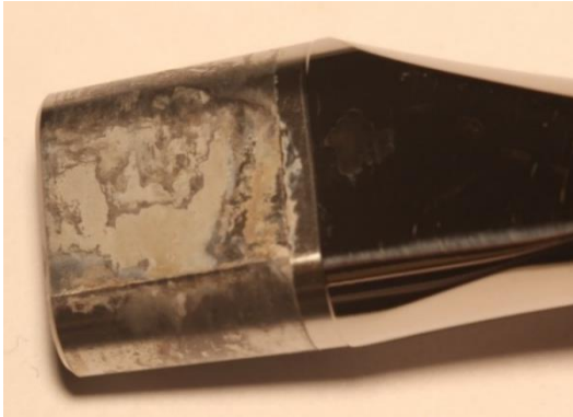
Figure 4.13: Advanced fretting associated with corrosion damage on the anterior surface of a hand-assembled CoCrMo neck following a fatigue test.
