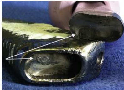
Figure 2.22: Image of an in vivo fractured long CoCrMo modular neck showing the fractured neck fragment inside the stem pocket [48].
