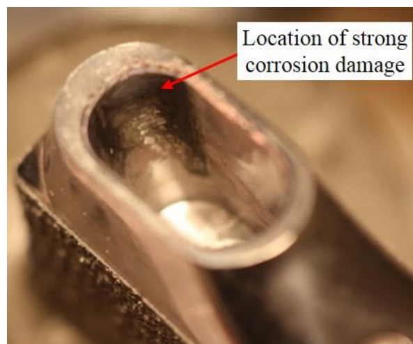
Figure 4.6: Corrosion (black debris) on the medial surface of a Ti6Al4V stem following a corrosion test with a hand-assembled CoCrMo neck.
