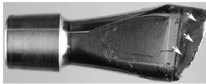
Figure 2.21: In vivo fracture of a long Ti6Al4V modular neck with the arrows pointing at the fretting and corrosion damage [4].
