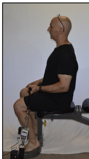
Figure 2. Apparatus to measure MVIC elbow flexor force production and SEMG amplitude for normalization for the biceps brachii.
