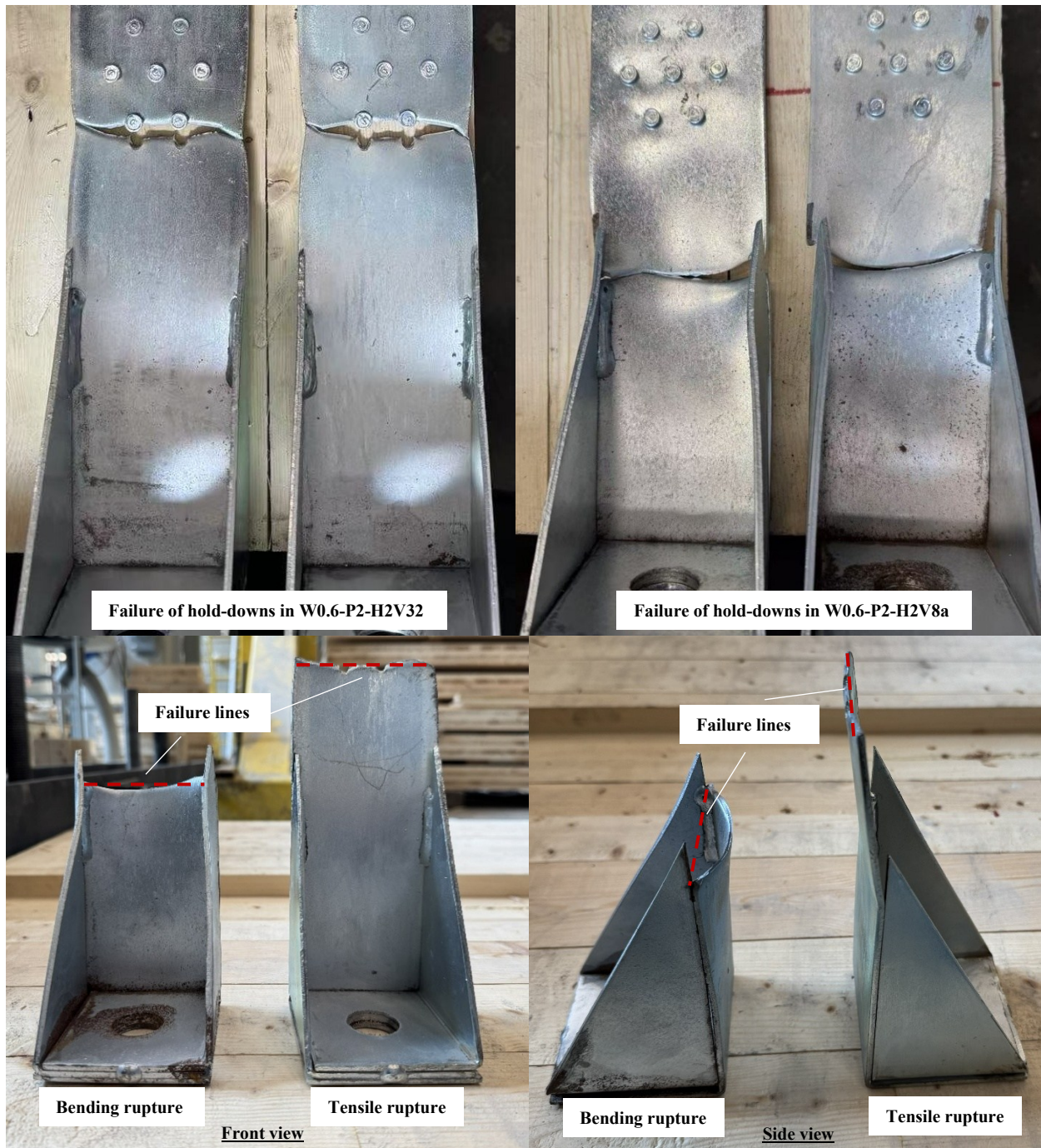
(a) Comparison of the rupture characteristics of hold-downs caused by tension and by combined tension and bending
