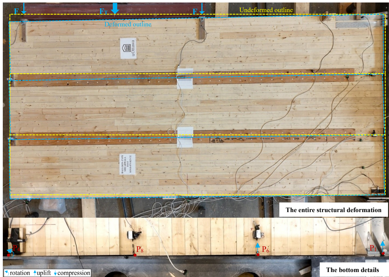
(b) Entire structural deformation and the bottom details of specimen W0.8-P3-H2V32 at the failure moment
