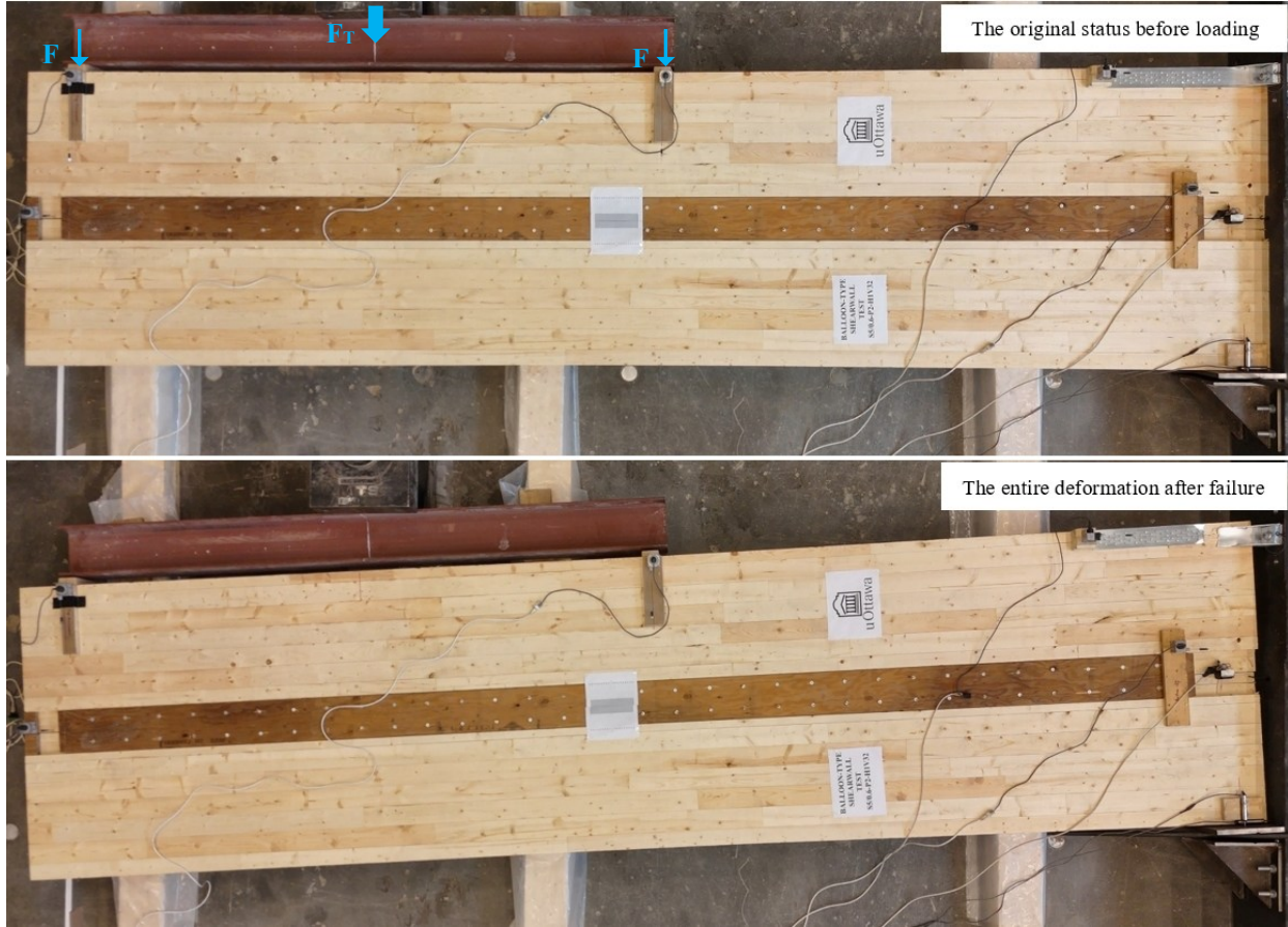
(a) Entire structural deformation of specimen W0.6-P2-H1V32
