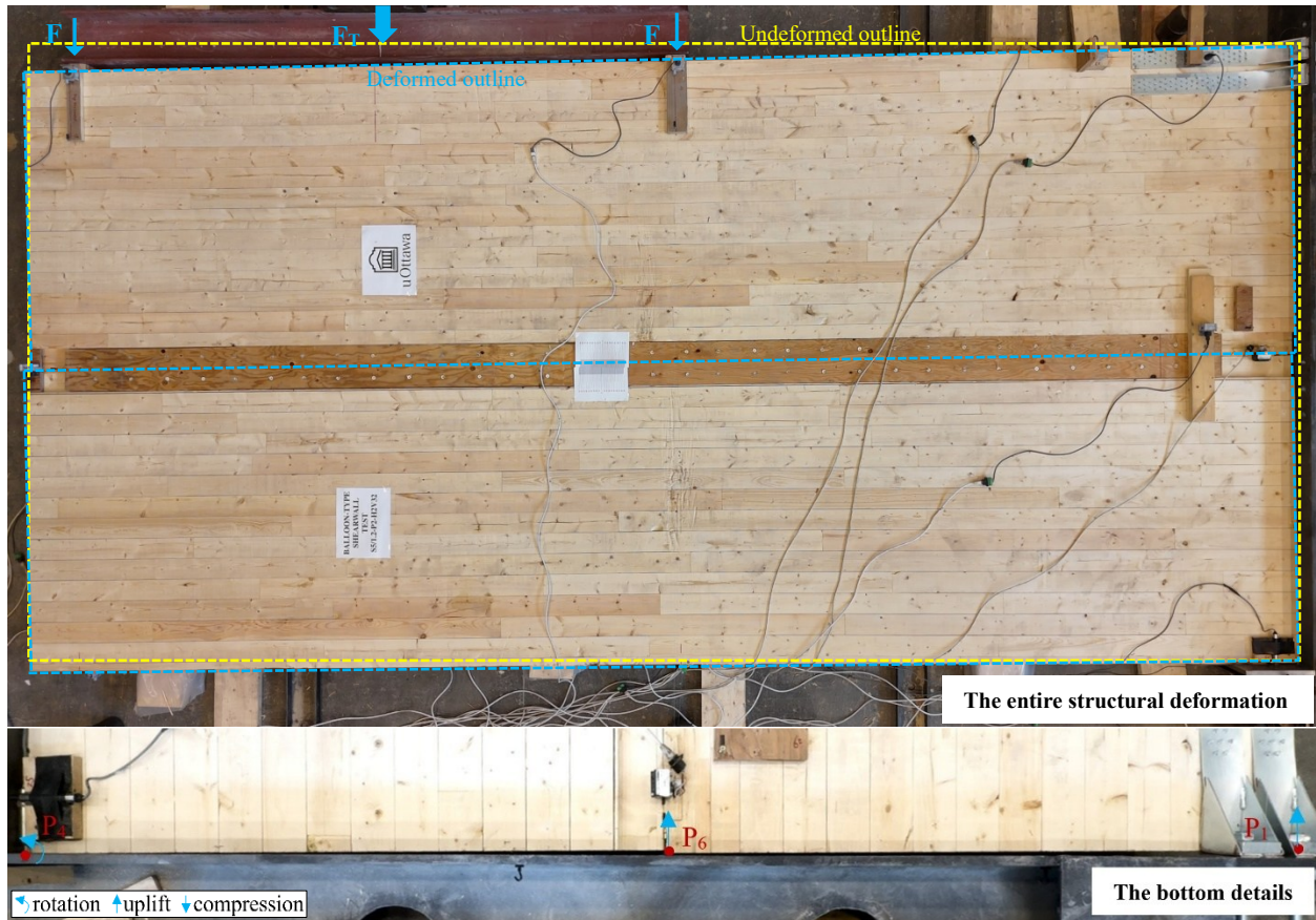
(c) Entire structural deformation and the bottom details of specimen W1.2-P2-H2V32 at the failure moment
