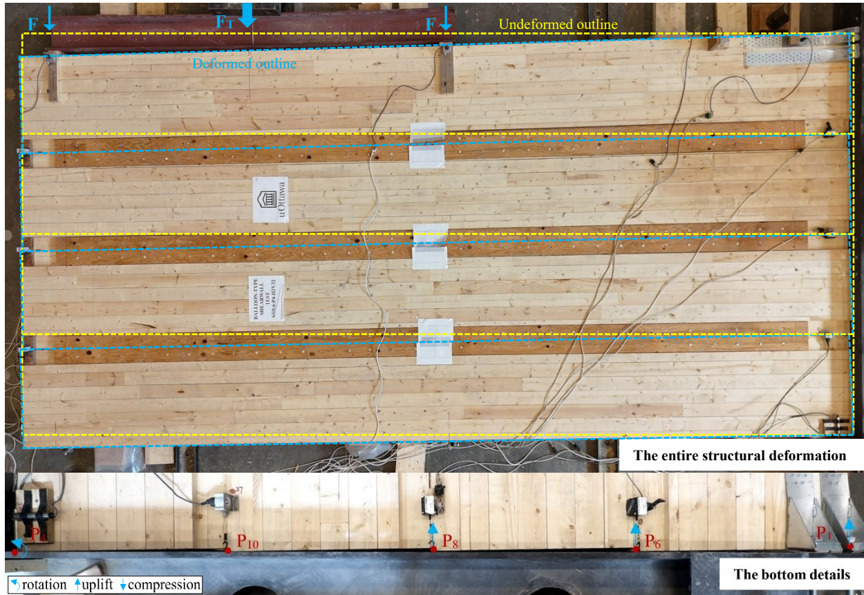
(a) Entire structural deformation and the bottom details of specimen W0.6-P4-H2V32 at the failure moment
