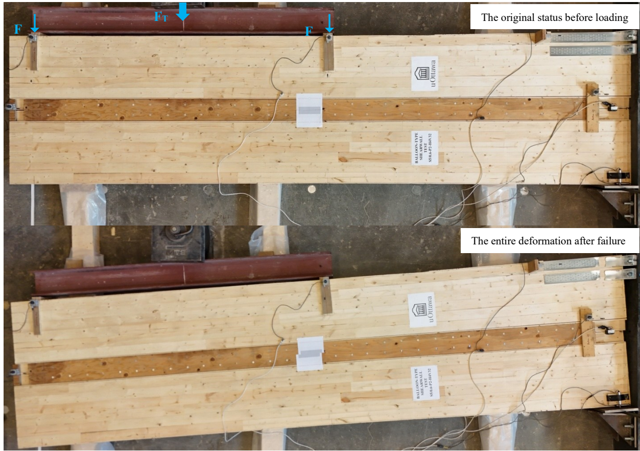
(c) Entire structural deformation of specimen W0.6-P2-H4V32
