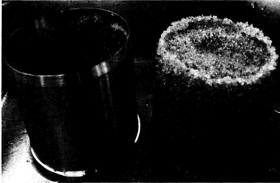
a. Self-standing Column of Saturated Ottawa Sand
