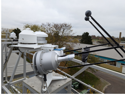
(a) DNI and DHI measurement
