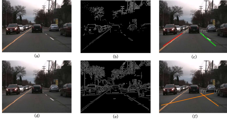
Figure 3.5: (a) and (d) are the same frame from Clip 4. (b) and (e) show the binarized picture of Sobel and Canny respectively. (c) is the final detection result of (b), while (f) is the result of (e).
