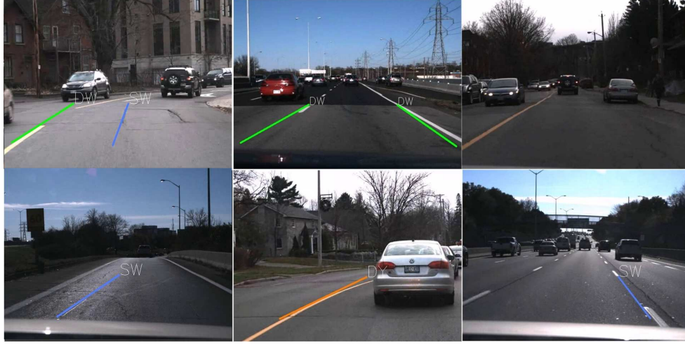
Figure 4.6: The left column shows false positive and false negative detection. The middle column shows false negative recognition for solid lines and false positive recognition for dashed lines (erroneously recognize solid as dashed line). The right column shows false negative detection and one erroneous recognition (recognize dashed line as solid).
