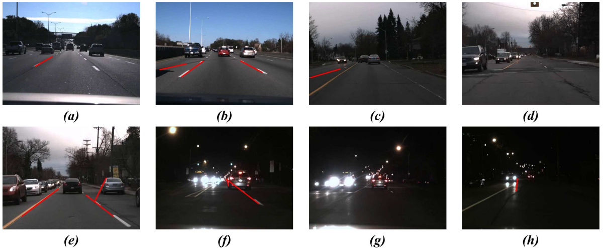
Figure 4.4: Examples of False Positive and False Negative results of simplified module: (b) and (e) show the false positive results as well as correct detection; (a) and (f) show the false negative results for one lane marking while the other one being correctly detected; (c), (d), (g) and (h) show the false negative results for both left and right lane markings as well as some false positive results.
