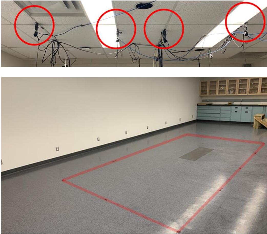
Figure 4.4 Physical setup of the four-camera arc layout. The top image slice shows the cameras arranged in the arc layout. The bottom image shows the virtual border of the hallway capture volume in red.
