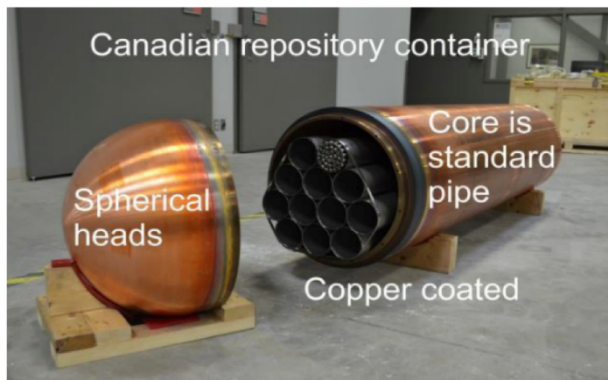
Figure 2.4 Mark II UFC proposed for use in NWMO DGR concept (from Dixon (2019))
