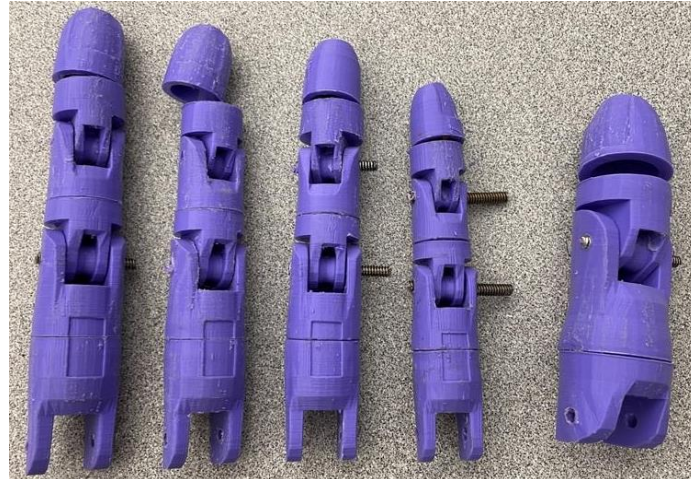
Figure 4.3 Printer and assembled fingers of Robo Twin with middle, index, ring, pinky and thumb from left are similar in size as that of an adult male
