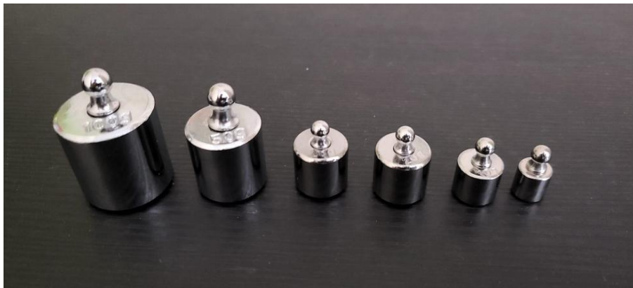
Figure. 4.14 Standard masses used to validate the calibration of FSR sensors
