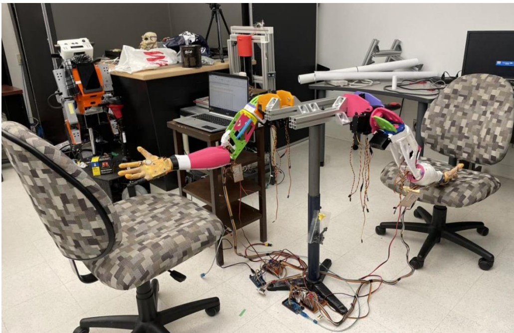
Figure 5.1 Robo Twin handshake experiment setup
