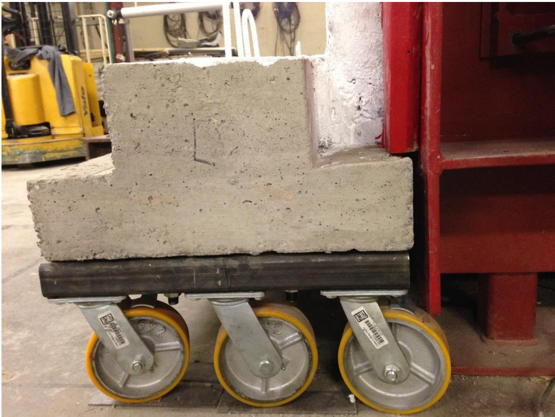
Figure 3.24 – Close-Up of Base Support System
