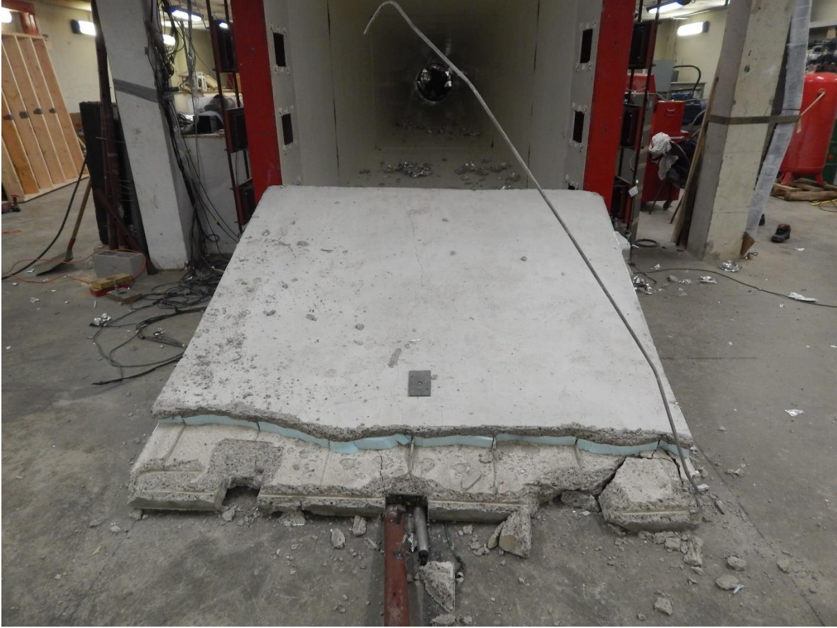
i) Complete failure of upper panel supports
