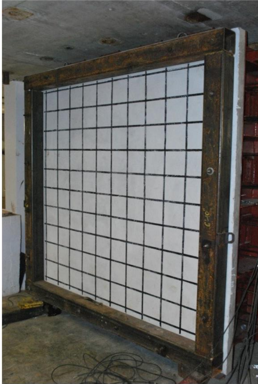
Figure 1.13 – E. Jacques Experimental Setup for Two-Way Specimens
