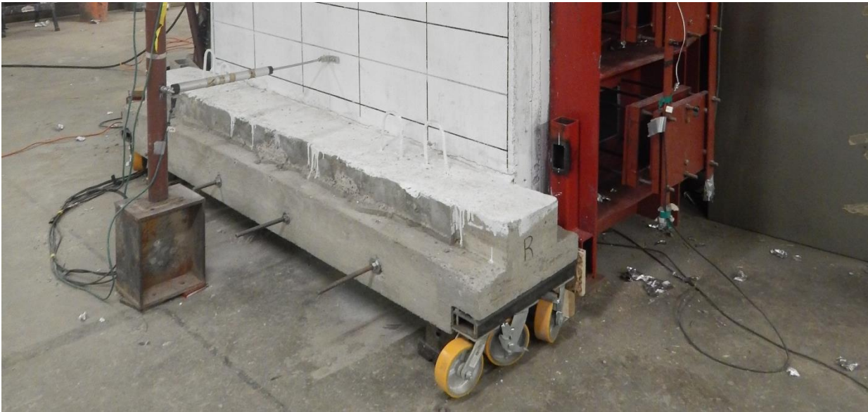
iii) Complete installation of panel with base connected to shock tube
