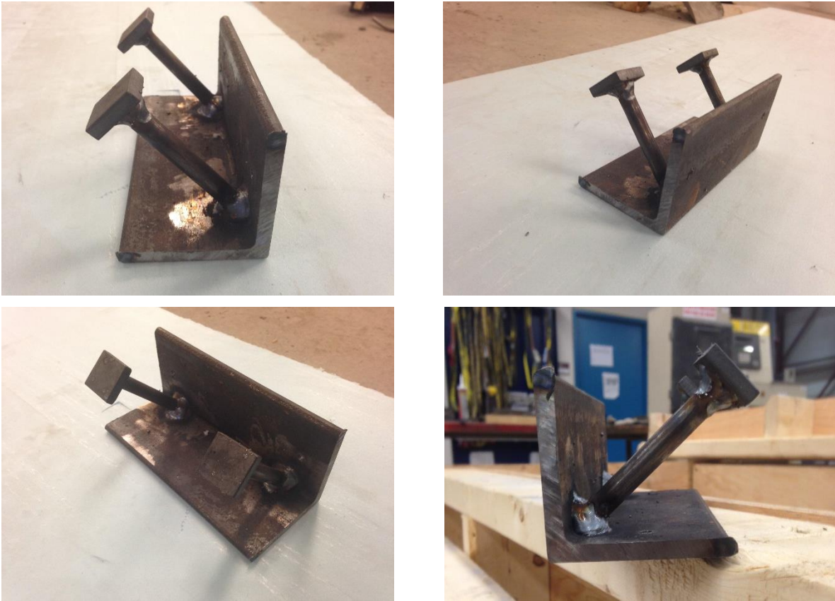
Figure 3.12 – Close-Up of Joist Seat (Upper Connection)
