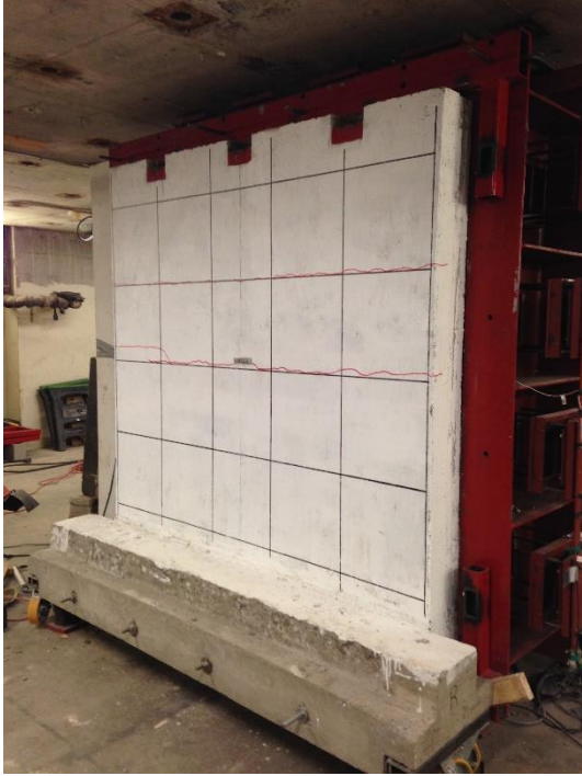
i) Test 1 – 72.4kPa & 57.9ms Prior to repair
