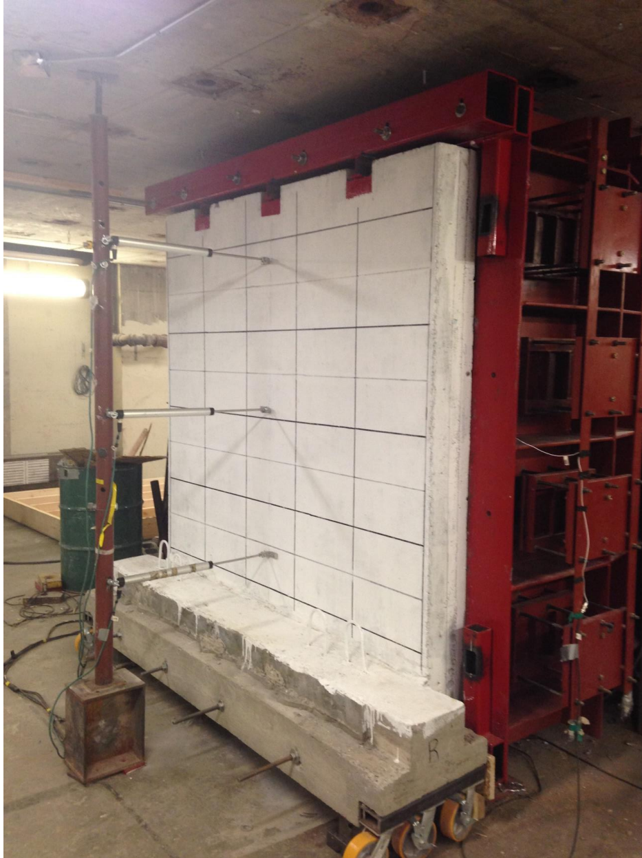
Figure 3.22 – Typical Test Setup for Sandwich Panel Series
