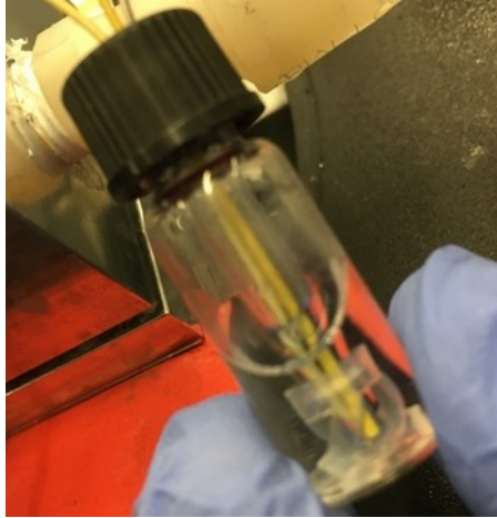
Figure 48: To fix settling an agitation mechanism was added, the pressure flow began in a separate vial filled with air, which then connected to the sample vial with PEEK tubing. Air bubbles in the sample vial led to agitation preventing settling.
