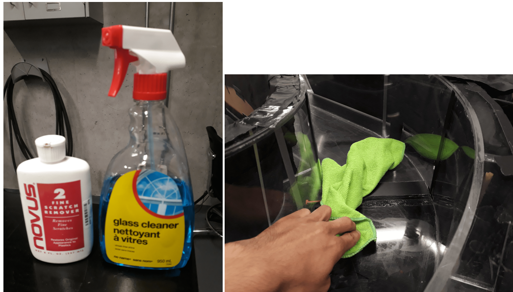
Figure 13: Products and motions to clean the walls
