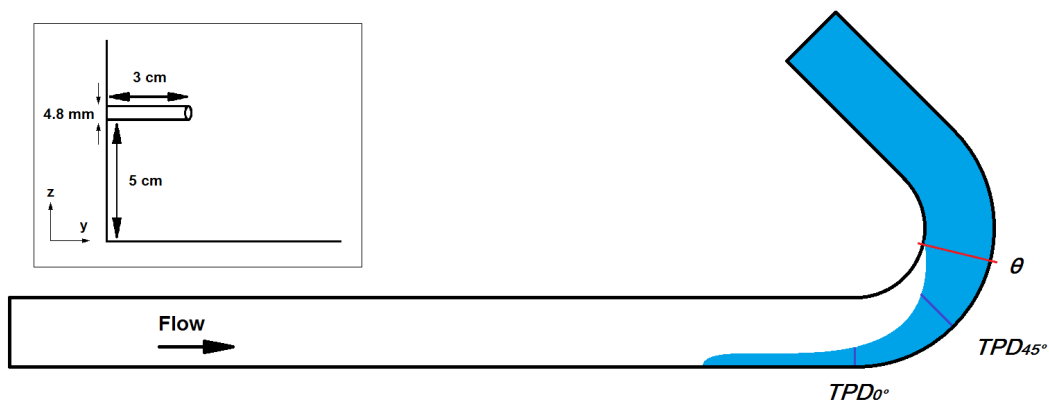
Figure 4.2: Schematic of jet and flume during dye test, showing definition of transition point distance, TPD , and opposite wall contact angle, \theta
