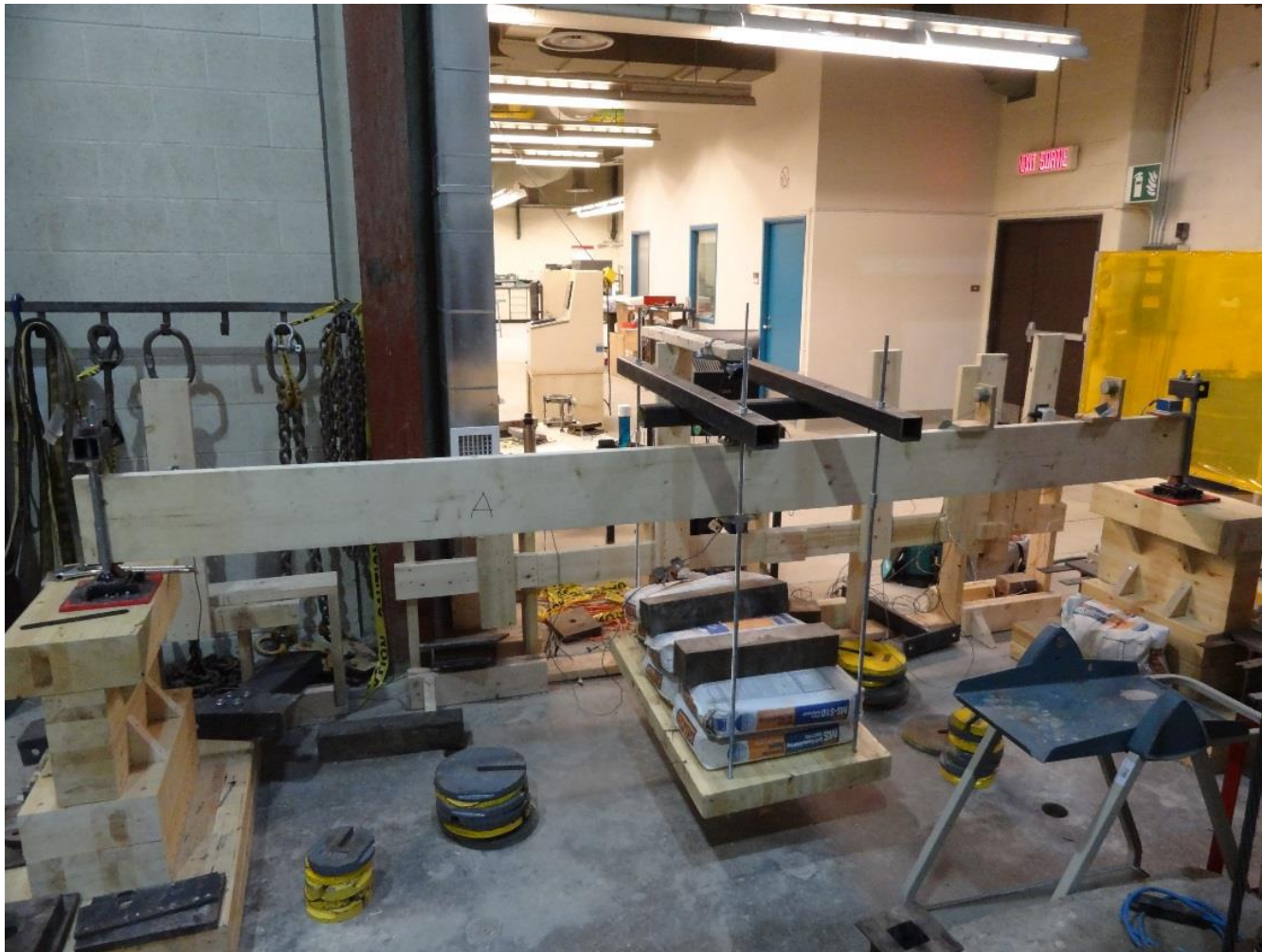
Figure 4.12 The set-up of lateral torsional buckling test
