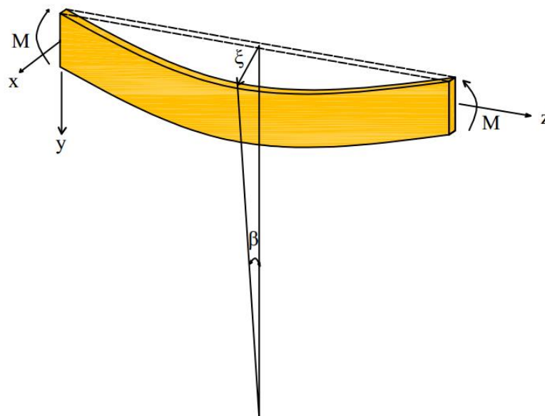
Figure 1.3 Lateral torsional buckling of beam
