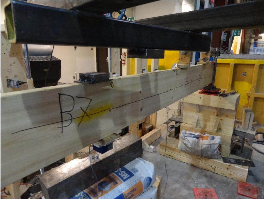
Figure 5.15 Failure mode by shear stress
