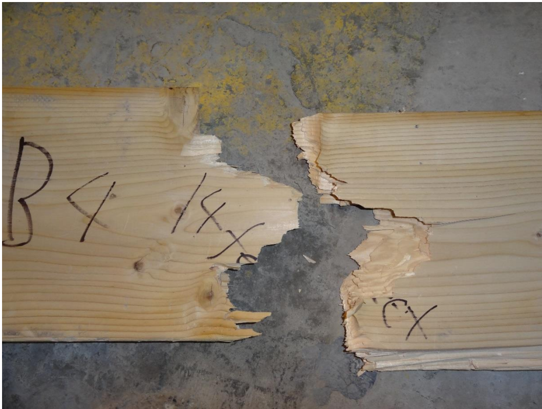
Figure 5.13 Failure mode with outside lateral surface under tension
