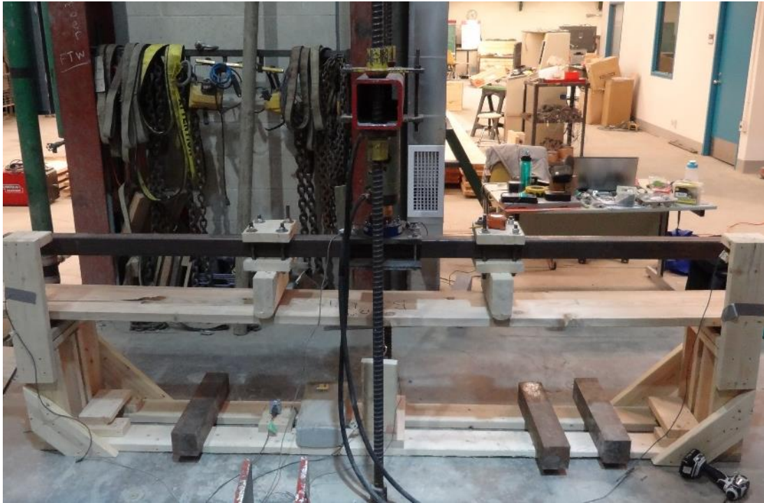
Figure 4.8 The set-up of weak axis bending for SPF
