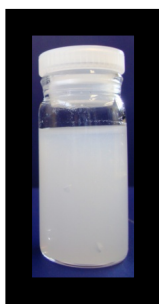
Figure 4.1 Example of a gel obtained in a successful solution polymerization of TEOS in the presence of Al in the aqueous solution
