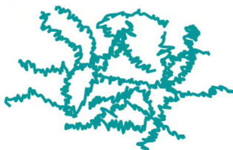
Figure 2.7 Gel structure under acidic condition (Nagarale et al., 2006)
