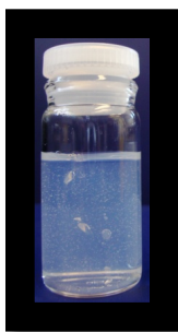
Figure 4.2 The gel obtained from polymerization of TEOS in the presence of hydrochloric acid-ammonium hydroxide
